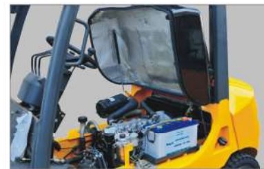
Engine cover with gas-filled cylinders and sound absorbing material.
