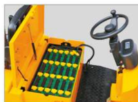
Large capacity batteries located in the lowest part of frame, offers low centre of gravity.
