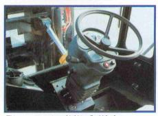
This new generation of Liftking Forklifts features a onepiece steering column with gauges and controls conveniently situated, leaving additional room in the operator's compartment.
