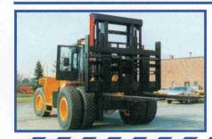
The LK43K features dual-front tires and a heavy duty roller mast.
