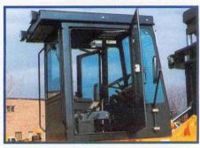
The LK43K is available with a two-door walk-through cab, complete with heater, defroster fan, windshield wiper, dome light, sliding window, lift-off removable doors and sound insulation.
