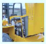
The P-Series forklifts offer a flip-up engine cover for easy access during maintenance
